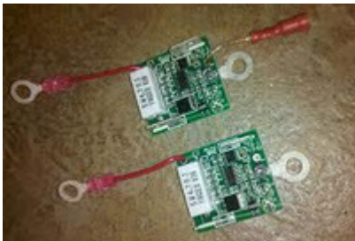
Typical Cell Mounted BMS
