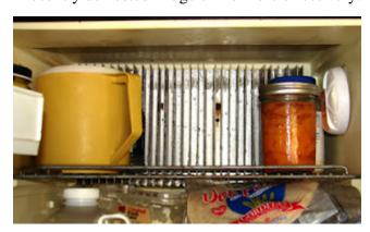
An RV refrigerator relies on natural convection to get the cold air moving around inside the refrigerator section, and you'll find the cold comes from those aluminum colored fins in the back, up near the top of the compartment. Open the door to take a look or grab something out, warm air from your living quarters invades that refrigerated space. Moisture in the air typically makes its way to those fins and attaches itself like a barnacle on the bottom of a ship.
